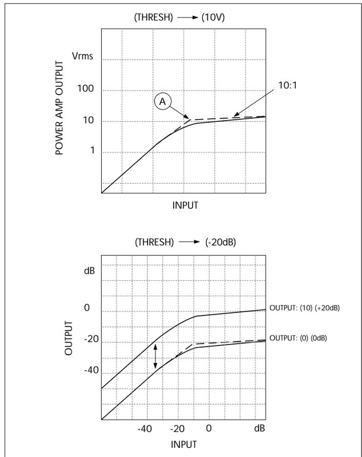
The top diagram shows the compression curve of the L-1102 in limiter (speaker protection) mode. Output amplitude is linear with respect to input, up to the threshold (A), and gentle and constant thereafter for compression in the ratio of 10:1. The bottom diagram (leveler) shows compression of an output signal when the input level exceeds a predetermined threshold. The effects of 0dB and +20dB output-level settings are also shown.
