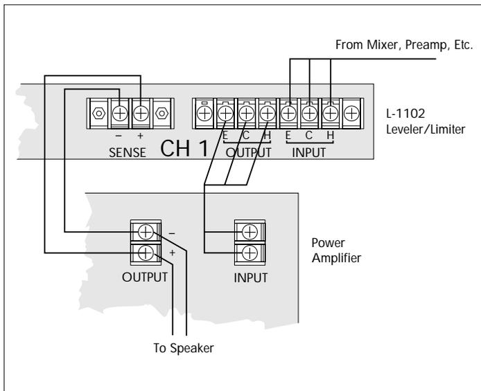
**Connections for limiter operation (one channel). The wires between the power amp's output and the L-1102's sense input are unnecessary when the unit is used as a leveler.**
