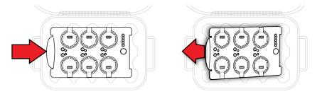
If batteries are already installed and require replacement, remove them. Then install new ones, being careful to match the batteries' direction to the polarities indicated by "+" in the battery holders.
