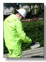
Survey meters measure radiation levels using the same radiation sensors employed in detectors and dosimeters. They are the oldest type of device discussed here, and look similar to traditional identifiers, but have a probe that's held in one hand, while the meter box is held in the other.
